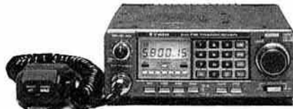
TRIO TR7930 Two metres FM mobile transceiver
